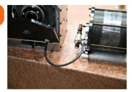
Mount pump to back of indexer using (2) cap screws (provided) Connect 1/4" hose from air inlet port side (as shown on back of cylinder)
