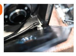
Insert bulkhead fitting (provided). Spread permatex around inside of flange on both sides (permatex provided)
