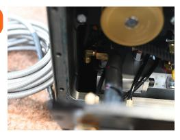
Locate 1/4" hose running from PORT 2 on solenoid valve to inside and near top of box running to inside of rotary 3
